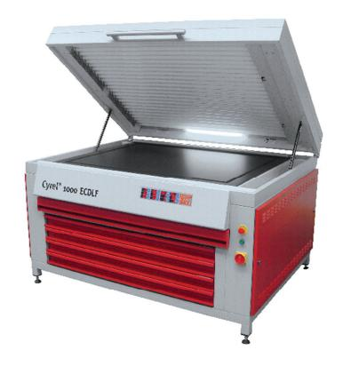
The four dryer drawers are located beneath the Light Finisher section. There is one timer per dryer drawer for regulating the temperature. Automatic blowers on both dryer drawers further control the set temperature. The exhaust air- flow is monitored by a safety sensor.
