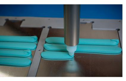
Thermally conductive polyurethane material is applied between EVs' battery cells and cooling plates to help control heat by maintaining thermal conductivity over an optimal temperature range.
