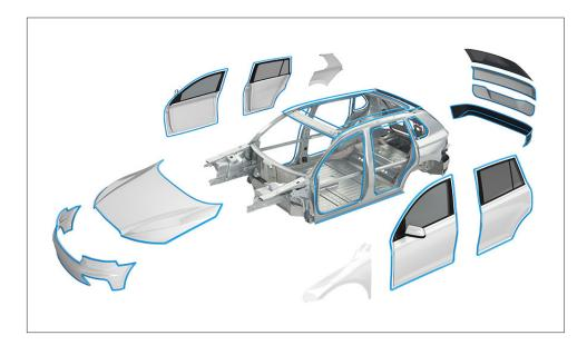
Structural and multi-material bonding adhesives add stiffness for durability and crashworthiness while also reducing vibrational energy for improved acoustics.
