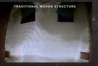
14 plies 600D (24x24) .50psf impacted with 9mm 124gr FMJ @ 955fps
