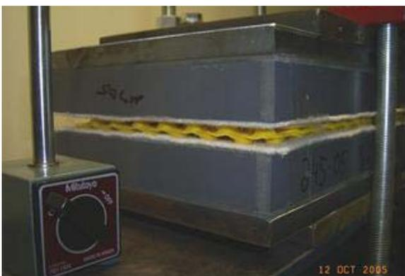
Figure 4. Drainage composite between soil boxes
