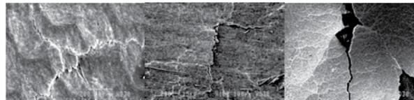
Some tested roof membranes crack quickly after exposure to UV and lose their watertightness. Microscopic pictures — scale 100x
